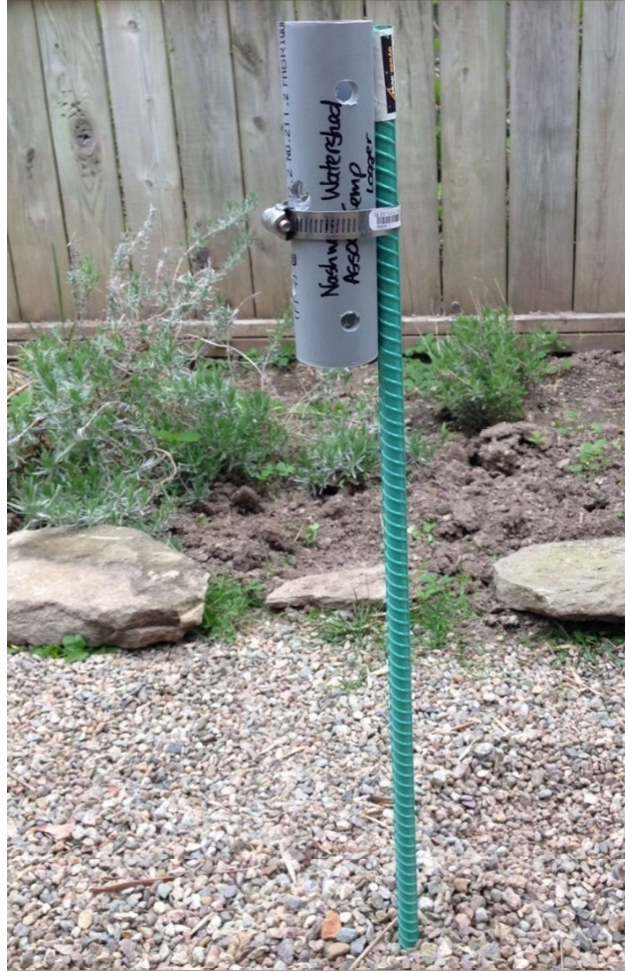
Figure 2. A logger in its casing prior to deployment. Zip ties were added for extra security.
